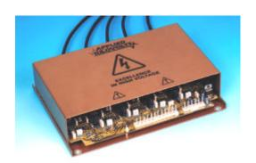
The 5x5 MS005MAA provides 5 separately controlled 0 to 5kV outputs, at up to  $300\mu A$ . Each one can be configured by the factory as positive or negative (combinations of polarity are possible e.g. 3 positive and 2 negative). Each channel is controlled by its own 0 to +10V control signal, and each has its own 0 to +10V monitor output. The module is powered from 24V DC, and draws 2 Amps fully loaded.
